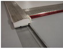
Extra sheet is placed next to the chain guide. It is a protection against sediment (result of the circulating transport chain)
