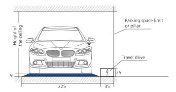
The platforms are guided by rails and are placed in front of traditional parking spaces.
