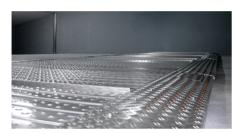
Platforms with side carriers and driving sheets made of trapezoidal sheet.
