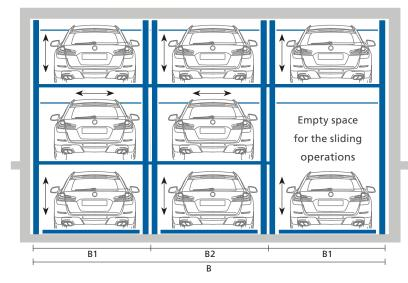
On the entrance level are sliding platforms with one empty space on the right (on the left: possible as an option). On the lower level the system is provided with lifting platforms. A lifting platform will be lifted or lowered to the empty space on the entrance level.
