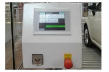
Operation by touch screen with key switch and emergency-stop. With brief operating instructions fastened on the wall and cabling to the power unit.
