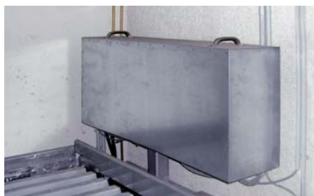
Sound insulation hood for the power unit
