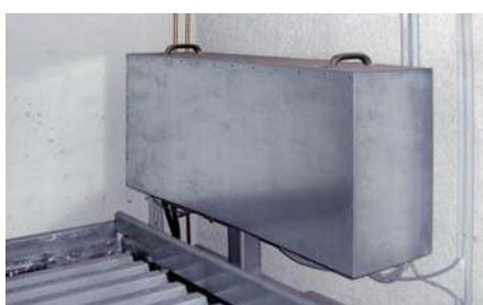
Sound insulation hood for the power unit
