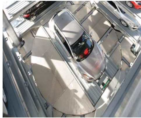
Vertical conveyor system with turntable
