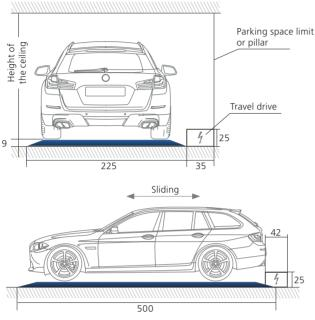
Load per parking space: max. 2.000kg, wheel load: max. 500kg. Optionally up to 2.300 kg or 2.600kg, wheel load max. 650kg. Heavier cars shall not drive over the sliding platforms.
