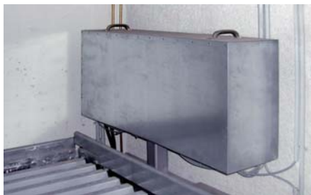
Sound insulation hood for the power unit
