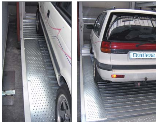
Catwalks Positioning on the left side of the parking space even more comfortable, when walking to the driver's door. 1,5mm zinc sheet, surface are coined. The catwalks are screwed to the driving plates, available with corrosion protection version "Classic" or "Classic Plus".
