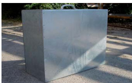
Sound insulation hood for the power unit
